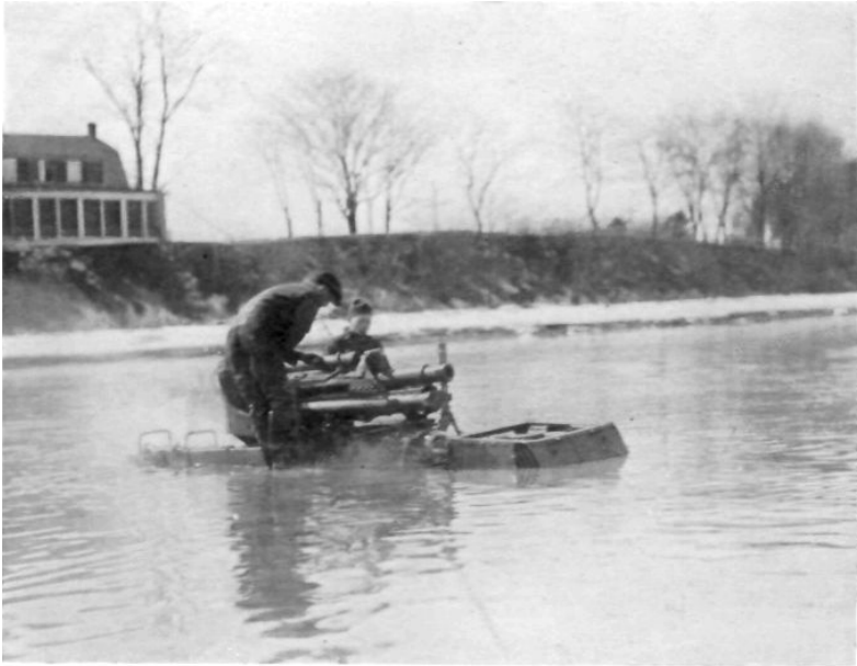
THIS PHOTOGRAPH TAKEN FROM A BOAT SHOWS THE MOTOR RUNNING WHEN ABOUT THREE-QUARTERS SUBMERGED.
