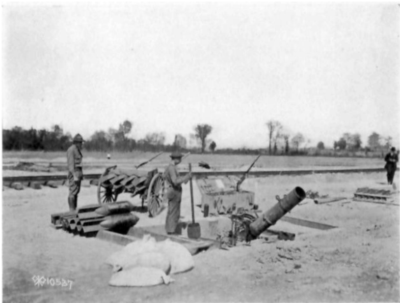
240 MM. TRENCH MORTAR—MARK I. OPEN SIGHT ATTACHED. SHELL CARRYING CART—LOADED TOOL BOX AND ACCESSORIES
