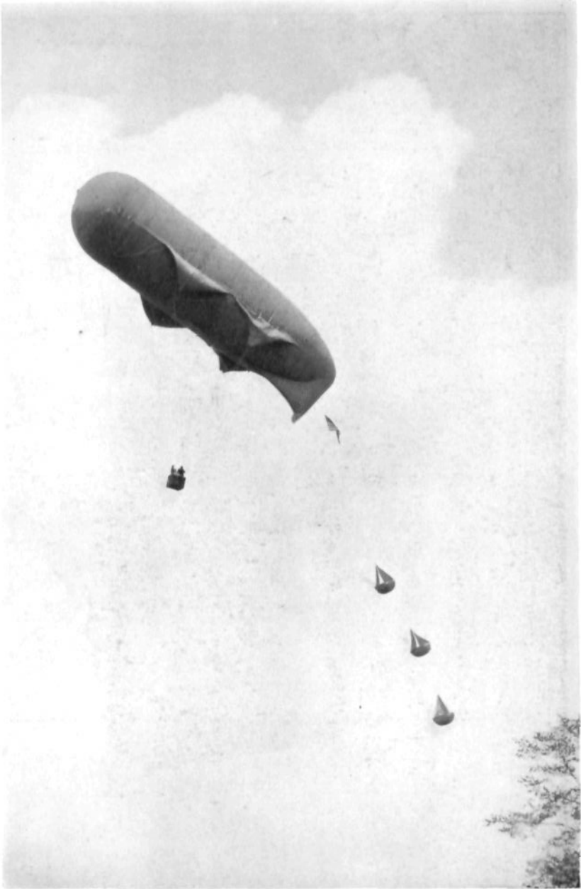
GOODYEAR KITE BALLOON SHOWING ARRANGEMENT OF TAIL CUPS
