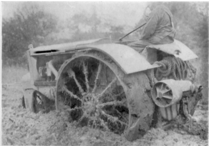
FIG. 14.—FIFTY-HORSEPOWER WHEELED TRACTOR STALLED WHILE ATTEMPTING TO PULL A 4.7-INCH GUN. THE POWERFUL ENGINE KEPT TURNING THE WHEELS WHICH SPUN AND DUG IN UNTIL THE BODY OF THE TRACTOR WAS RESTING ON THE GROUND.
