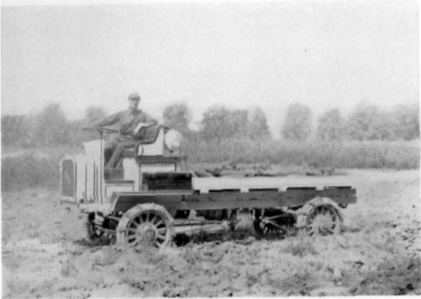
FIG. 5.—A THREE-TON FOUR-WHEEL DRIVE TRUCK WITH FULL LOAD RUNNING ON PLOWED GROUND WET BENEATH THE SURFACE. WHEELS ARE CUTTING ABOUT THE INCHES.
