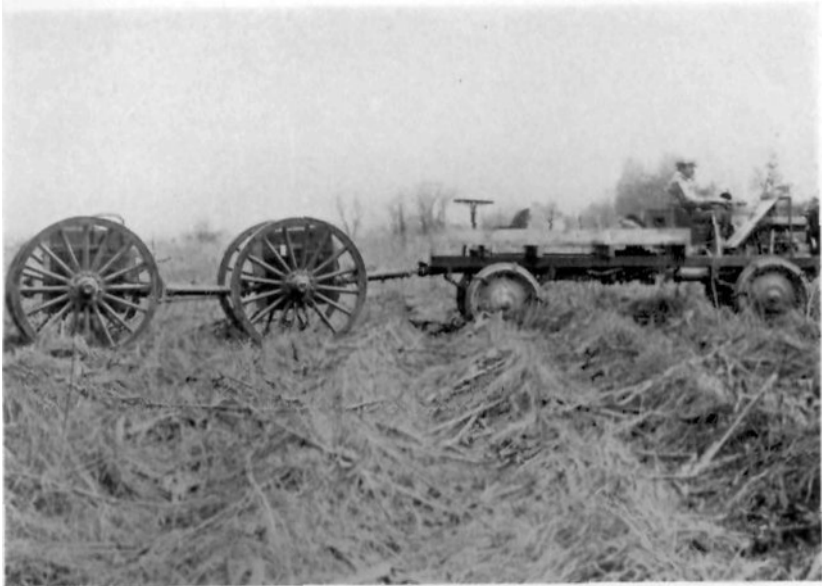
FIG. 9.—TWO-TON FOUR-WHEEL DRIVE TRUCK TOWING LIMBER AND CAISSON OVER CORN FIELD WITH DEEP FURROWS.
