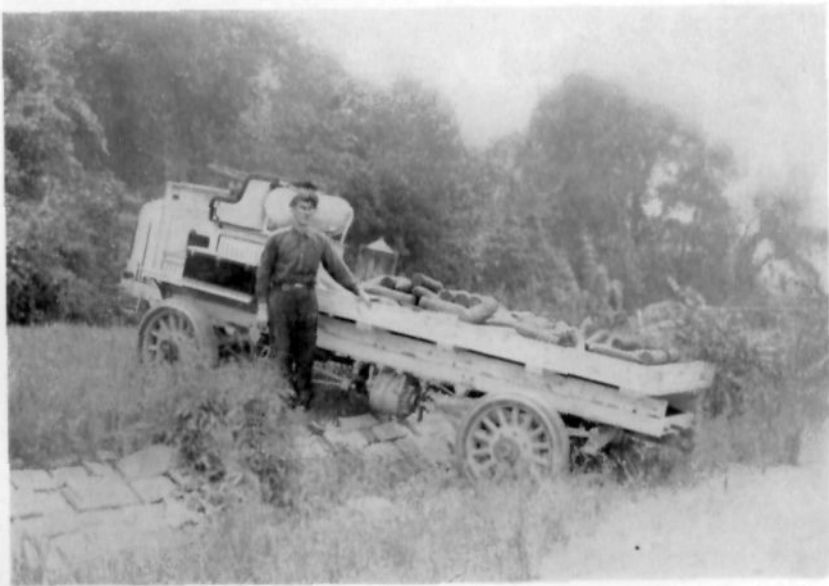
FIG. 6.—THREE-TON FOUR-WHEEL DRIVE TYPE OF TRUCK CROSSING DITCH. UNDER SUCH CIRCUMSTANCES A TWO-WHEEL DRIVE TRUCK WOULD MERELY PUSH ITS FRONT WHEELS AGAINST THE SIDE OF THE DITCH. THE FRONT WHEELS OF THE FOUR-WHEEL DRIVE BEING POWER WHEELS CLIMB OUT.
