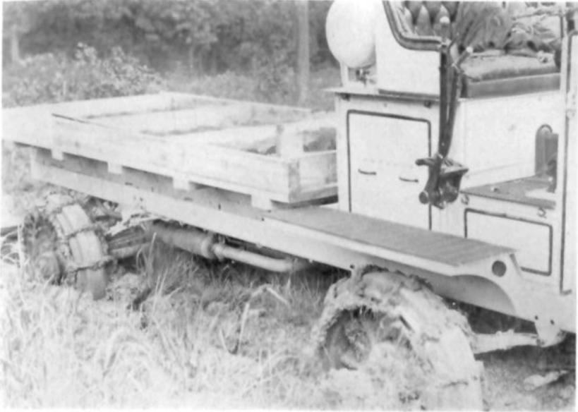
FIG. 7.—ABOUT THE ONLY KIND OF GROUND THAT WILL STOP A FOUR-WHEEL DRIVE TYPE—MUD SO DEEP THAT THE WHEELS SINK UNDER THEIR OWN WEIGHT UNTIL AXLES REST ON GROUND.
