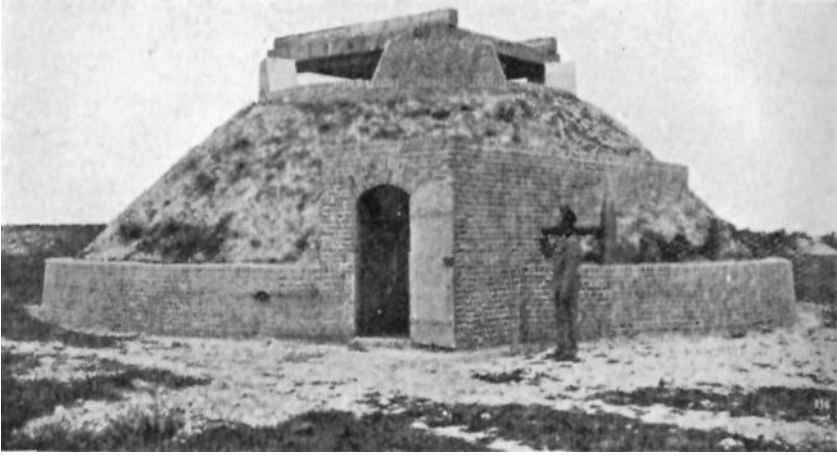
PROVING GROUND OF THE SCHNEIDER WORKSHOPS AT HOC. ARMORED BURSTING PITS FOR TESTING EXPLOSIVE SHELLS
