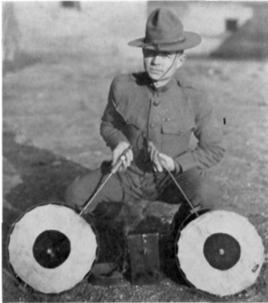
SHOWING DETAILS OF FLAGS AND NIGHT CONNECTIONS, NOTICE SWITCH BUTTON ON FLAG HANDLE IN RIGHT HAND OF OPERATOR
