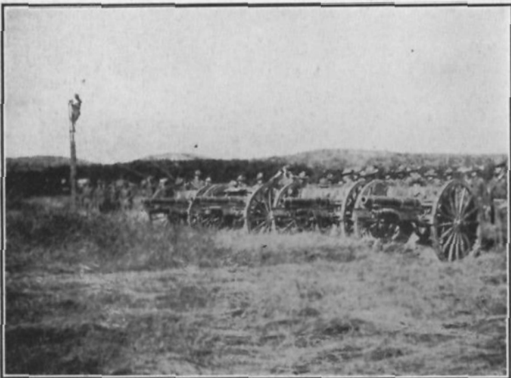
This photograph shows the position of the guns for firing, with one foot interval between pieces. This formation gives a dispersion which corresponds to service conditions for mid-artillery ranges. The observation ladder was found useful in picking up difficult targets and in recording results of fire.
