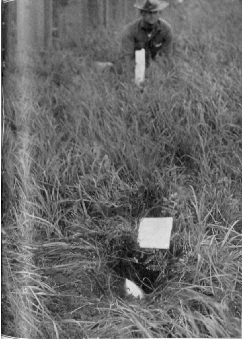
PHOTO 20. UNEXPLODED H. E. SHELL FROM 4.7-INCH GUN; MAN KNEELING AT POINT OF ENTRANCE.
