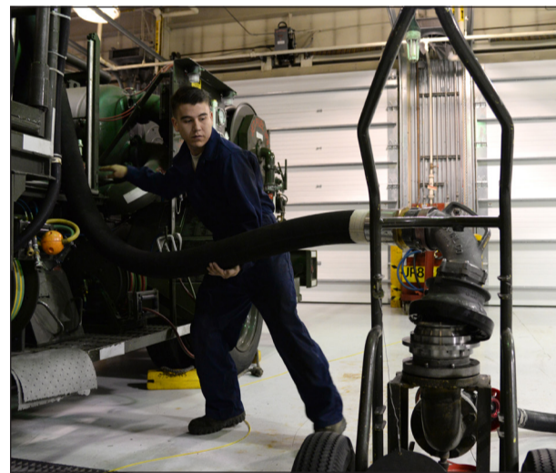
U.S. Air Force Senior Airman Steven Venegas, a 354th Logistics Readiness Squadron firefighting and refueling vehicle and equipment maintenance journeyman, hooks up a fuel pump, Sept. 10, at Eielson Air Force Base. Venegas needs the pump put together in order to perform troubleshooting procedures while completing routine maintenance on the truck. (Photo by Airman 1st Class Cassandra Whitman)
