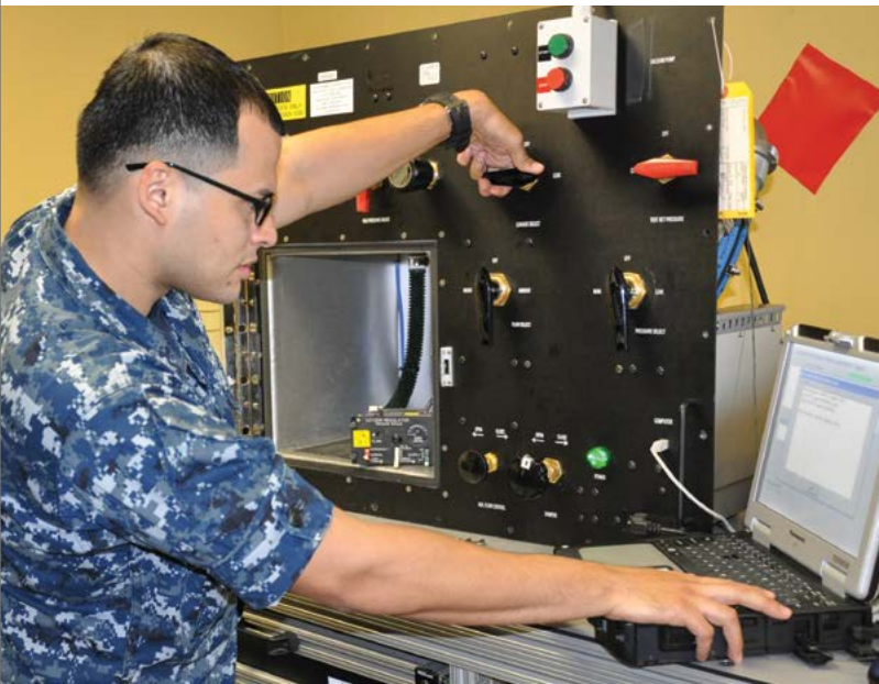
▲ Aircrew Survival Equipmentman 2nd Class Yithzack Licona tests crew oxygen regulators for a C-130 Hercules aircraft at Fleet Readiness Center Mid-Atlantic Detachment Washington. (U.S. Navy photo by Gary Younger)
