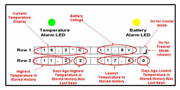
Figure 7. Schematic of the LED indicators and LCD display.
