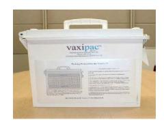
PXC (+7°C) must be chilled at 3°C (±1°C) for 24 hours.
