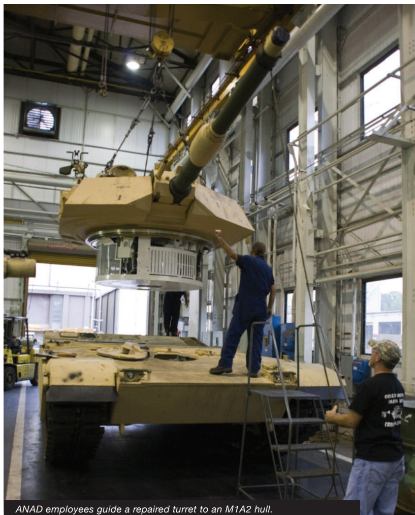
ANAD employees guide a repaired turret to an M1A2 hull.
