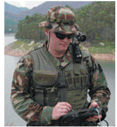
Right, NPS operations research student Ensign “Red” Miller on the ground in Thailand during COASTS-06 with a Kestrel shoulder-mount camera, ruggedized 802.11g portable computer, and Deny-GPS, a precision inertial navigation system that allows his position to be calculated in a non-GPS environment. Data on Miller’s position were relayed via an 802.11 wireless mesh network into the common operating picture viewed by officers in the Tactical Operations Center and other connected command centers.
