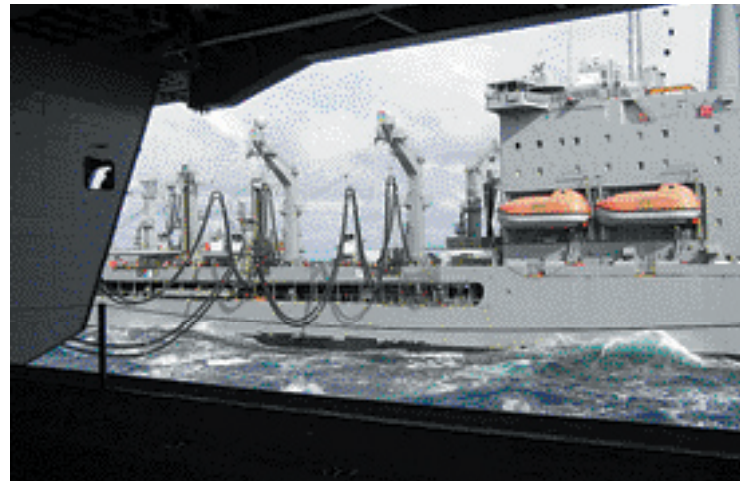
July 21, 2006 – View from the hangar bay of the USS Eisenhower, Military Sealift Command oiler USNS John Lenthall (T-AO 189) alongside the Eisenhower during an underway refueling.
