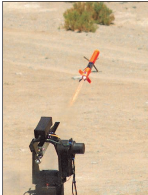
A forward-firing miniature munition known as Spike is launched during a successful counter-UAV demonstration on the land range at Naval Air Warfare Center Weapons Division China Lake. Spike was conceived, designed, developed and tested at NAWCWD. Since Spike is government-owned, the NAWCWD team can quickly modify the system to meet specific requirements. U.S. Navy photo by Patrick Kreidt
