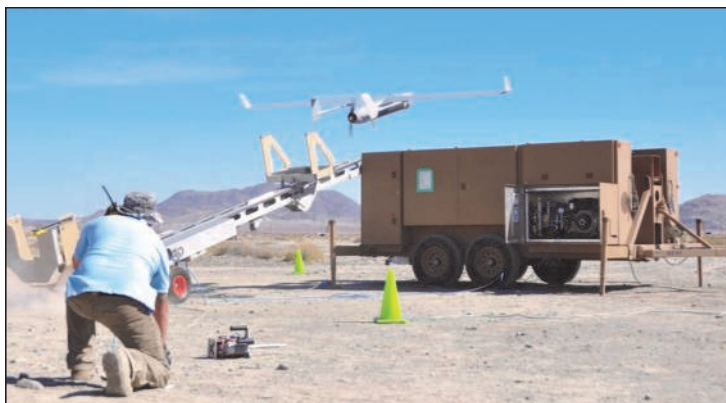
A rail launch is performed during Integrator unmanned aerial vehicle testing at Naval Air Warfare Center Weapons Division China Lake. U.S. Navy photo
