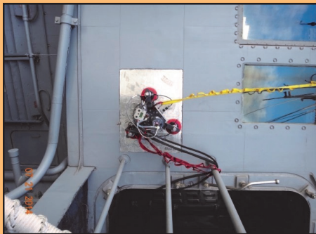
DoS Probe performing a measurement on CG-64 (USS Gettysburg).
