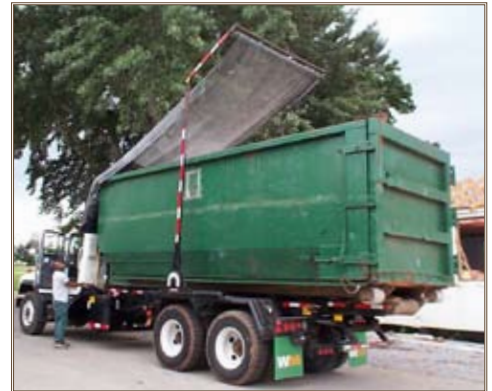
At Fort Campbell, Ky., a worker operates a waste container that has rollers at the bottom so it can be left onsite to collect C&D waste. After use, the container is rolled onto the truck's tilt bed and hauled away. Photo courtesy of Stephen Cosper, ERDC
