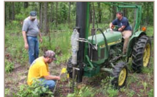
Soil core samples are collected using hydraulically operated coring equipment. Photos courtesy of Michael Hargrave, ERDC-CERL
