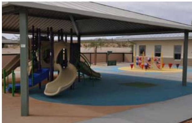
The playground equipment at Fort Irwin's newly completed CDC is made of recycled materials, including the spongy flooring, which used to be tennis shoes. Photo by Elizabeth Casebeer
