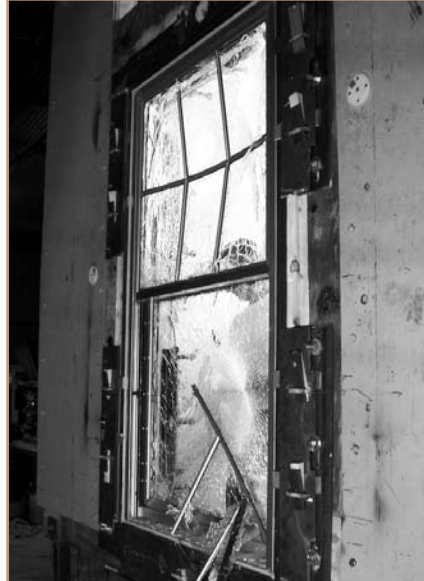
After blast testing of this hung window specimen, despite a small tear in the laminated glazing interlayer, no large glass fragments entered the reaction structure, so the window passed the test. Photos courtesy of U.S. Army Corps of Engineers.
