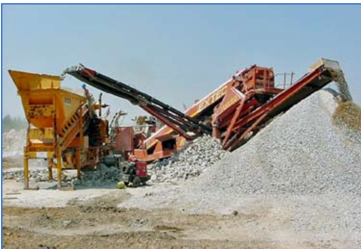
A concrete crusher at Fort Bragg reduces chunks of concrete debris into football-sized pieces that can be recycled for use wherever rock is needed on post. Photo courtesy of Sid Williamson
