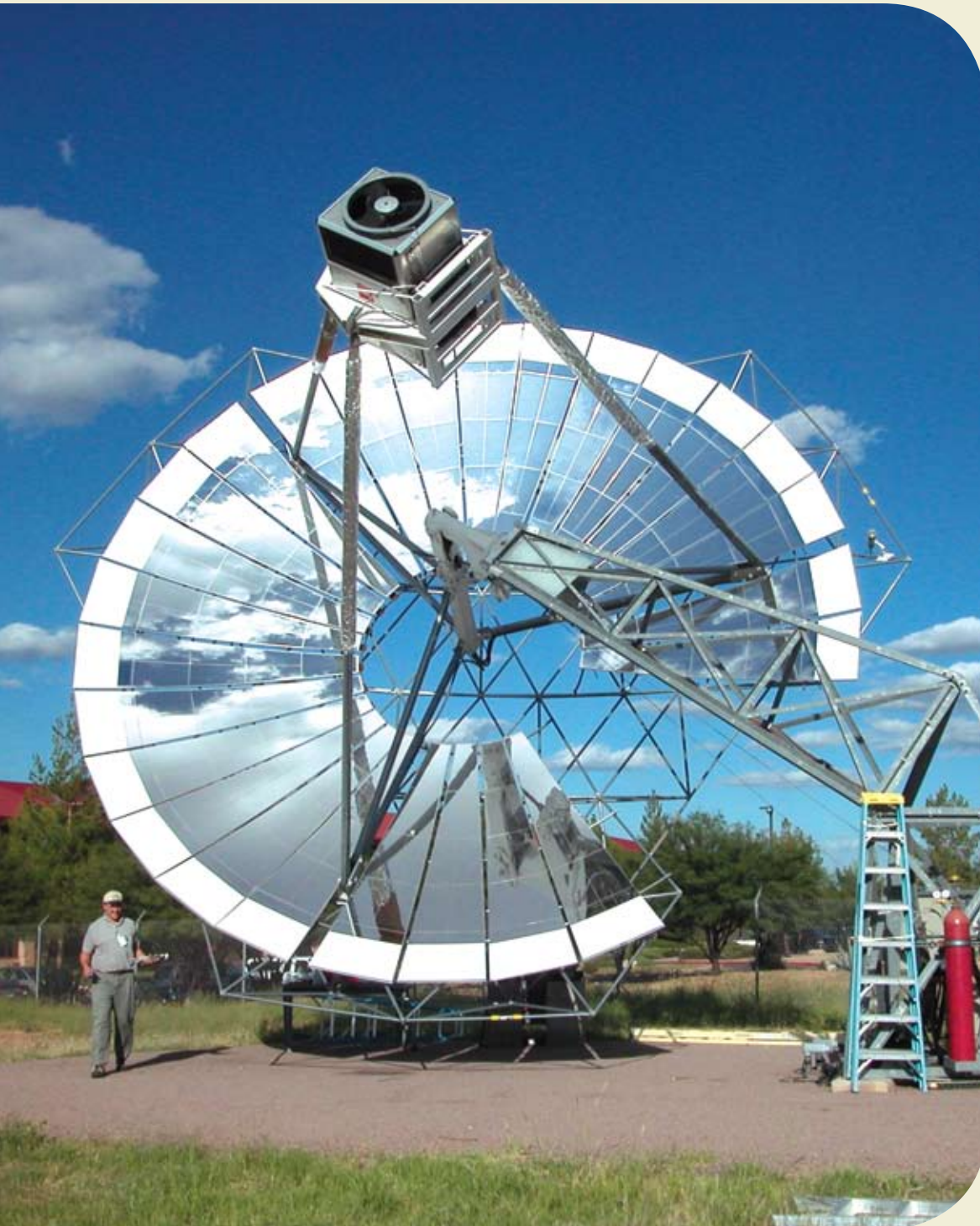
Chuck Andraka of Sandia National Laboratories is dwarfed by the dish/Stirling at Fort Huachuca, Ariz. Photo by Rich Diver, Sandia National Laboratories. Page 14
