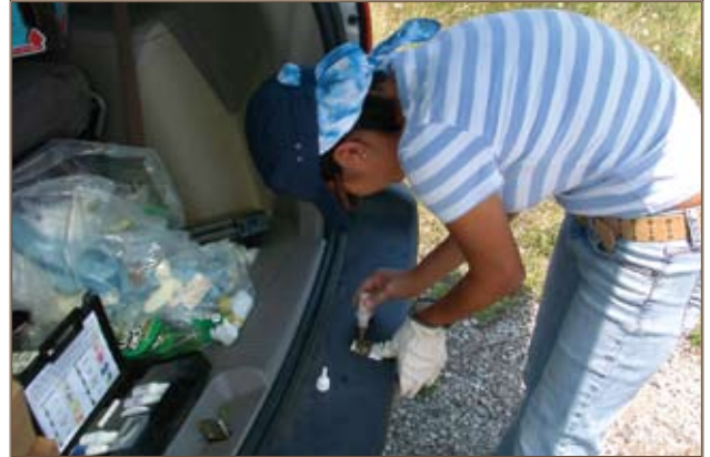
Field test technologies are often the best alternative for providing the user with a quick accurate response. Here, a field test kit is used to determine the presence of explosives in a soil sample. U.S. Army Engineer Research and Development Center photo
