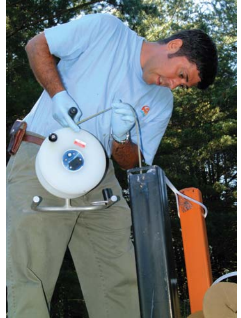
Brian Mailet, staff scientist with Arcadis G&M, Inc., measures the depth of water in a monitoring well on Fort Gordon, Georgia.
