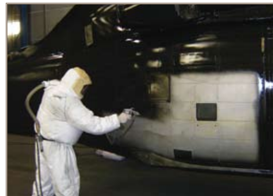
A painter applies a chromium 3 primer to a Blackhawk helicopter. Photo by Paul Simmons
