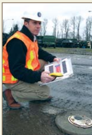
Jim Arnold collects location coordinates of a groundwater monitoring well with a handheld Global Positioning System unit. Photo by Mary Jane Jacobsen
