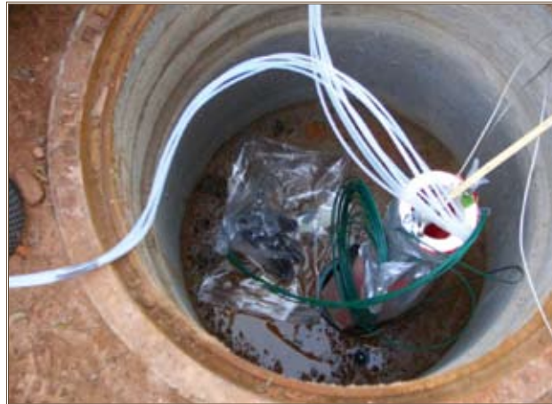
Permanent measuring devices were used in the groundwater monitoring wells at USAG Kaiserslautern. Photo by Uwe Dannwolf
