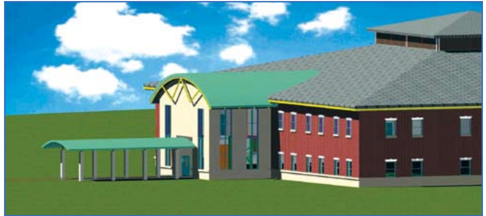
Building Information Modeling allows users to graphically view a final rendering of a building based on previously entered design criteria. Graphic courtesy of U.S. Army Corps of Engineers, Savannah District
