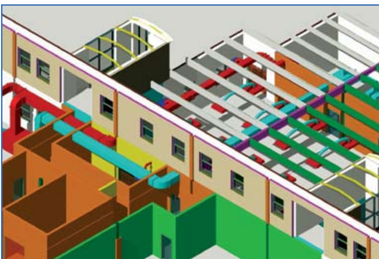
Using Building Information Modeling, designers are automatically notified if two objects, such as an air conditioning duct and piping, interfere with each other. Graphic courtesy of U.S. Army Corps of Engineers, Savannah District
