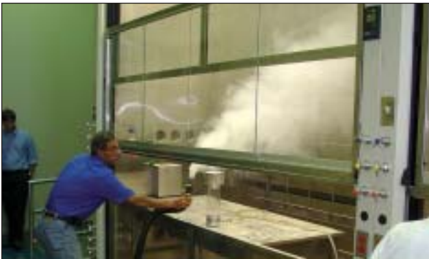
State-of-the-art, custom-designed chemical hoods and ultra-efficient carbon filtration banks are demonstrated. The safety and environmental control of the lab are critical to ensure that personnel and the environment are protected against lethal materials that are on the order of 600 times more toxic than industrial chemicals.
