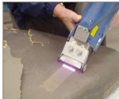
A handheld laser is used to remove the topcoat from a helicopter component at Fort Rucker, Ala. Photos courtesy of ARL
