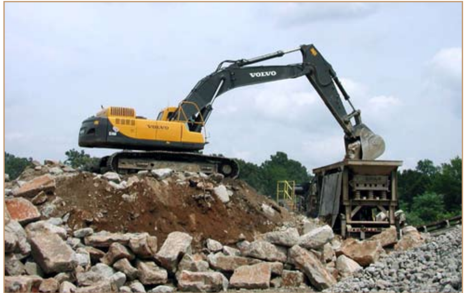
Concrete debris is recycled at Fort Campbell, Ky. Photo by Tom Napier
