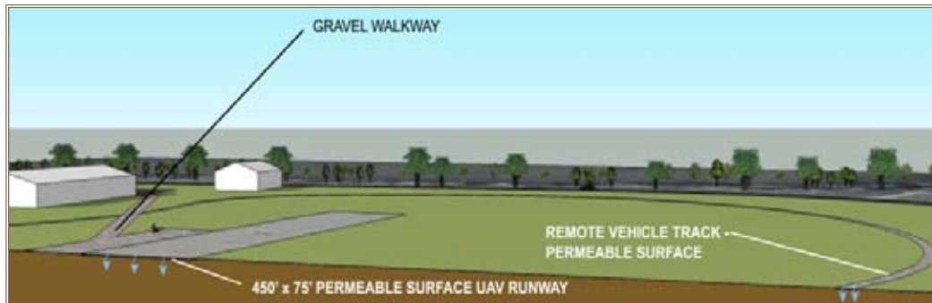
A LID plan uses permeable surfaces that allow water to filter through them. Graphic by Neil Weinstein, Low Impact Development Center, Greenbelt, Md.
