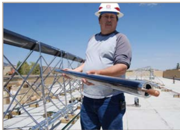
Craig Hansen, acting energy coordinator at Fort Huachuca, holds a double-wall evacuated solar tube that absorbs more heat with less radiated losses. Photo by Lee Roberts
