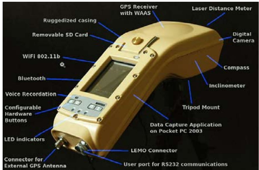
The hand-held device carries data that is invaluable in a contingency environment.
