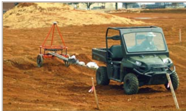
An EM-61 pulled behind an all-terrain vehicle is used during the geophysical investigation at Fort Campbell. Photo by Eric Cheng, Louisville District, U.S. Army Corps of Engineers
