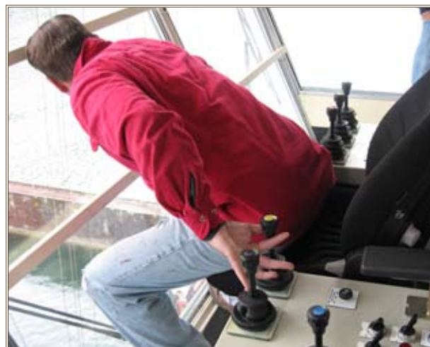
A dam crane operator must lean forward and twist in his seat to see the lift gates while groping for the controls, a situation that a systems safety analysis of the design would have spotted. Photo by Dave Stanton, Portland District, USACE
