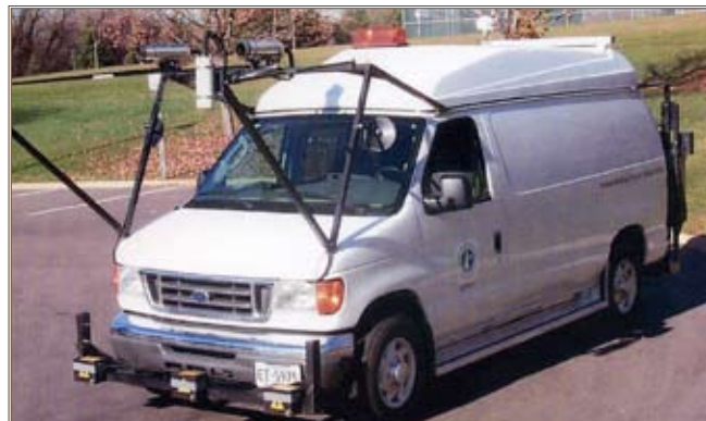
The distress data for PAVER is collected using a specially equipped vehicle. Photo courtesy of Minnesota Department of Transportation
