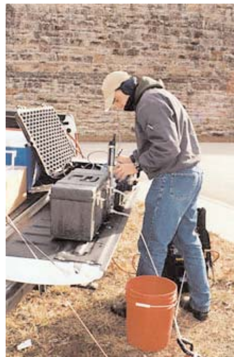
Scott Rose, an environmental scientist with Arcadis, measures the field parameters such as temperature, pH and clarity of groundwater from a monitoring well at Fort Leavenworth, Kansas. Under a performance-based contract, Arcadis is using a new in-situ technology to enhance and speed up the removal of contaminants in the groundwater at Fort Leavenworth. Cheese Whey and Molasses compounds are being used to augment carbon sources in the groundwater to enhance the biodegradation of volatile organic compounds or past contamination caused by the dry cleaning facility in the old United States disciplinary barracks at Fort Leavenworth.
