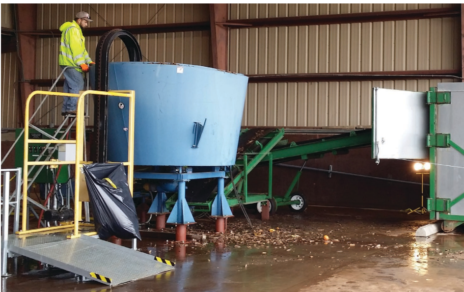
An employee mixes and loads feed stocks into the composting vessel. Photo by Audrey Oxendine.
