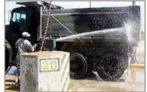
A Soldier cleans a truck at the Fort McCoy, Wis., CVWF, which has an 11-million gallon holding pond and recycles 98 percent of the water to clean equipment. U.S. Army photo
