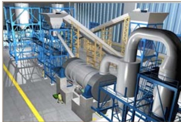
CERL's net-zero support includes a project to evaluate waste-to-energy options, such as this conceptual graphic of a rotary kiln waste gasification system now under construction at the Center for Environmental Science and Technology, State University of New York. Graphic courtesy of W2E Ventures Inc.
