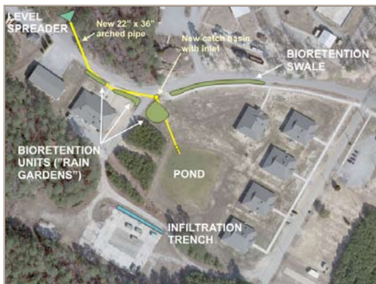
An overview of the Fort Lee training area LID project depicts the layout of LID techniques that increased areas for infiltration as opposed to the previous ditched areas that simply transferred runoff to the creek system. Graphic by Richard Stanford
