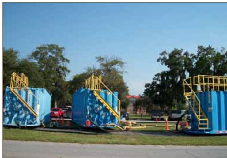
Eosine, fluorescein and rhodamine solutions are injected from 21,000-gallon tanks into the deeper zone of a trichloroethylene plume to trace the dispersion radius during a corrective actions feasibility study at Fort Stewart.
