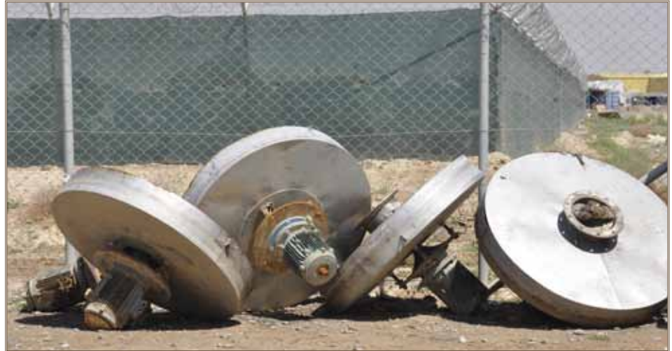
These four aerators await disposal after they were replaced as an upgrade to the Afghan National Army's Joint Regional Training Center wastewater facility. Photo by Karla Marshall
