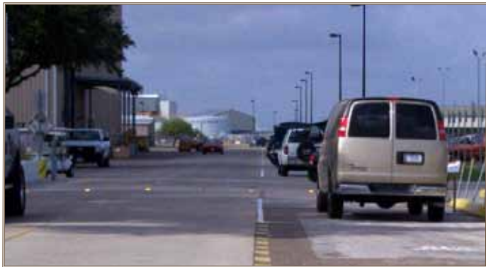
LED lights embedded in the pavement are activated when a pedestrian enters the crosswalk at a CCAD intersection. Photo by Daniel Cirilo
