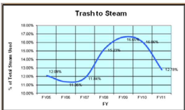
Fort Detrick uses municipal and medical waste to produce steam. Graphics courtesy of Fort Detrick
