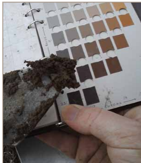
Soil color is determined using a Munsell Book. Photo courtesy of Construction Engineering Research Laboratory
