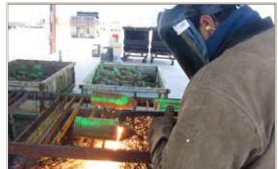
At Fort Irwin, a 90mm projectile is demilitarized before the metals are separated and sold as scrap. Photo by Versar Inc.
