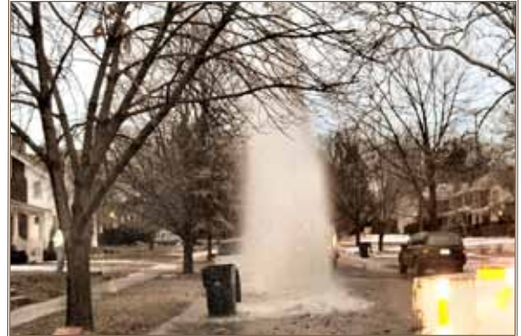
Catastrophic loss of water from main breaks like this one can be prevented with distribution system audits to locate and repair water leaks. Photo courtesy of City of Columbus, Ohio
