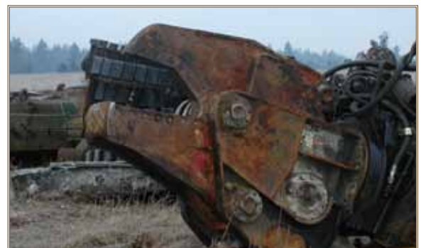
At Joint Base Lewis-McChord, shears are used to cut tank tracks and other smaller pieces. Photo by Billy J. Allen
