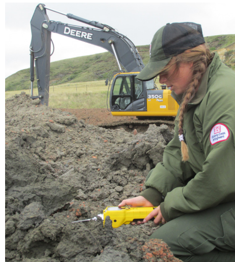
Hattie Payne, Natural Resource Specialist, tests soil for petroleum contamination. (Hanson, Petro-Hunt L.L.C.)
