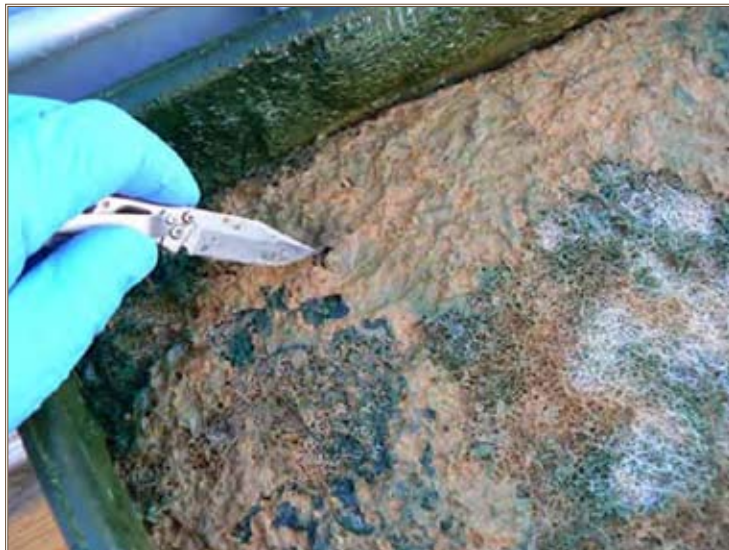
A pilot scale study at Fort Hood revealed that high levels of iron in the leachate saturated the biomats. Photos courtesy of ERDC
