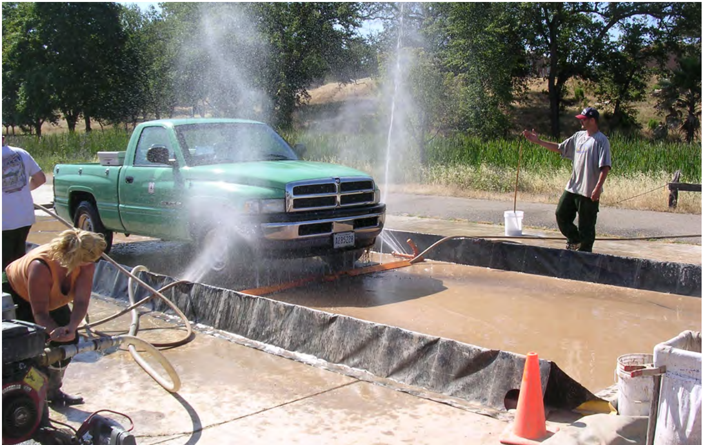
The U.S. Forest service developed an undercarriage washing system to clean vehicles that may have traveled through invasive species areas to minimize spread to other areas. (H. Balbach)
