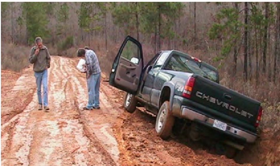
A team surveying road maintenance is caught when their 4WD truck slipped off the (possibly too-high) slick clay crown into a too-deep roadside ditch. (M. Sharif)
