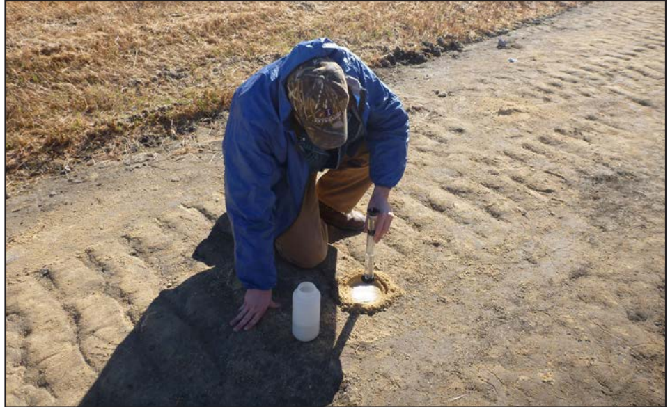
An infiltration test is conducted prior to biomedica and planting installation, incorporating an underdrain bioswale approach for stormwater management at Fort Hood, Texas. (U.S. Army Photo)
