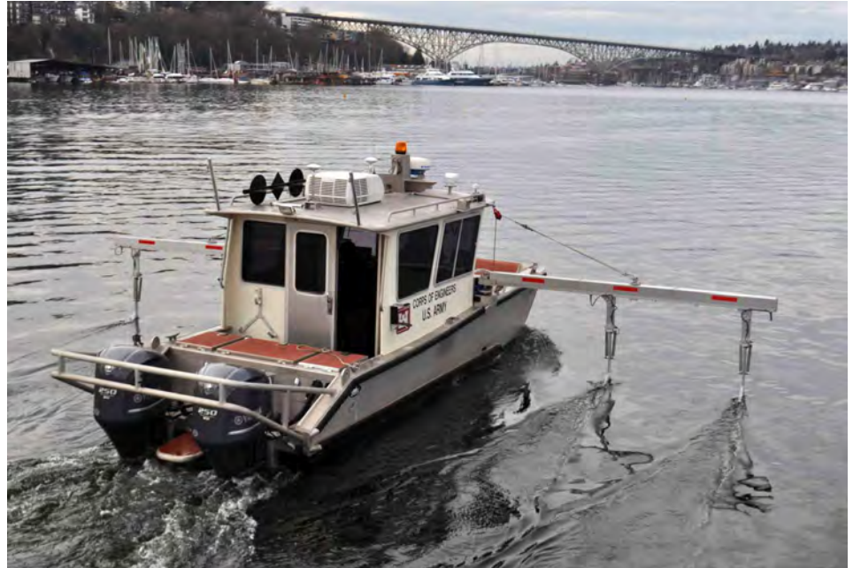
The 26-foot RGV-1 Munson boat undergoes a sea trial after being retrofitted with the Ross Sweep System. The vessel, equipped with a drop gate on the bow, can run a sweep-type survey along channels and single beam surveys when weather prevents deployment of the sweep booms. The Galveston District acquired this vessel in March to assist with its survey mission along the Texas coast. Photo by Sandra Arnold
