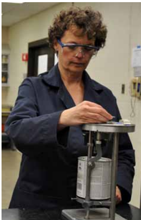
PTC Director Susan Drozdz measures paint viscosity in the laboratory at Champaign, Ill. Photo by Dana Finney
