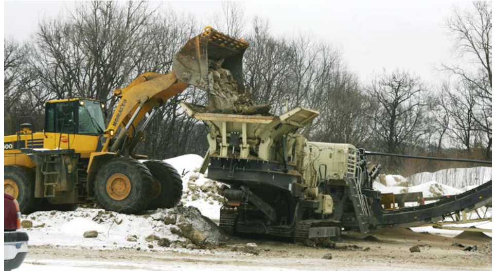
A contractor uses a loader to fill a rock crusher at an area on Fort McCoy's North Post. (Photo by Scott T. Sturkol)
