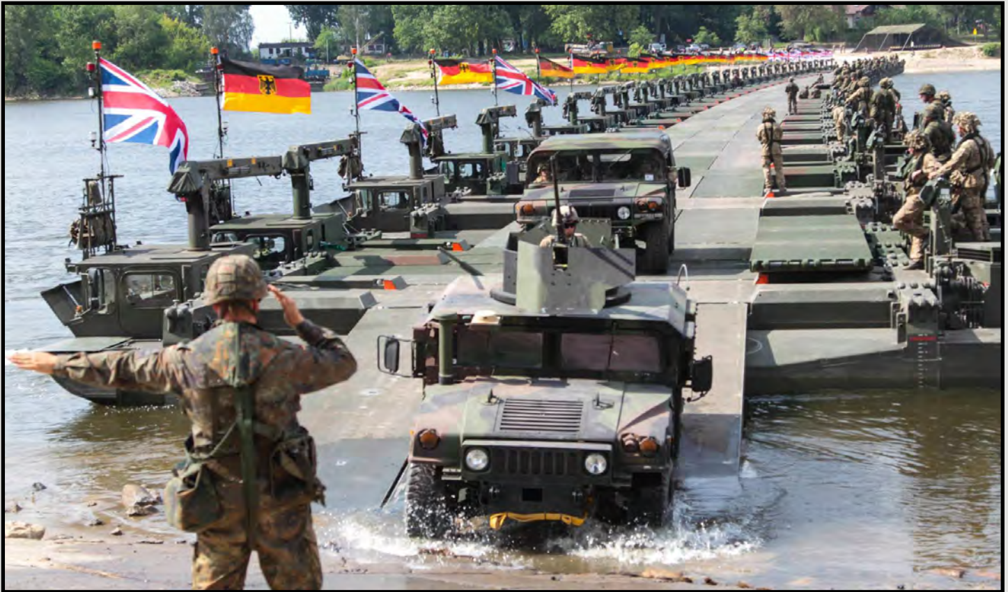
U.S. Soldiers drive vehicles over an M3 bridge during a water crossing mission conducted as part of Anakonda 16 in Poland.
