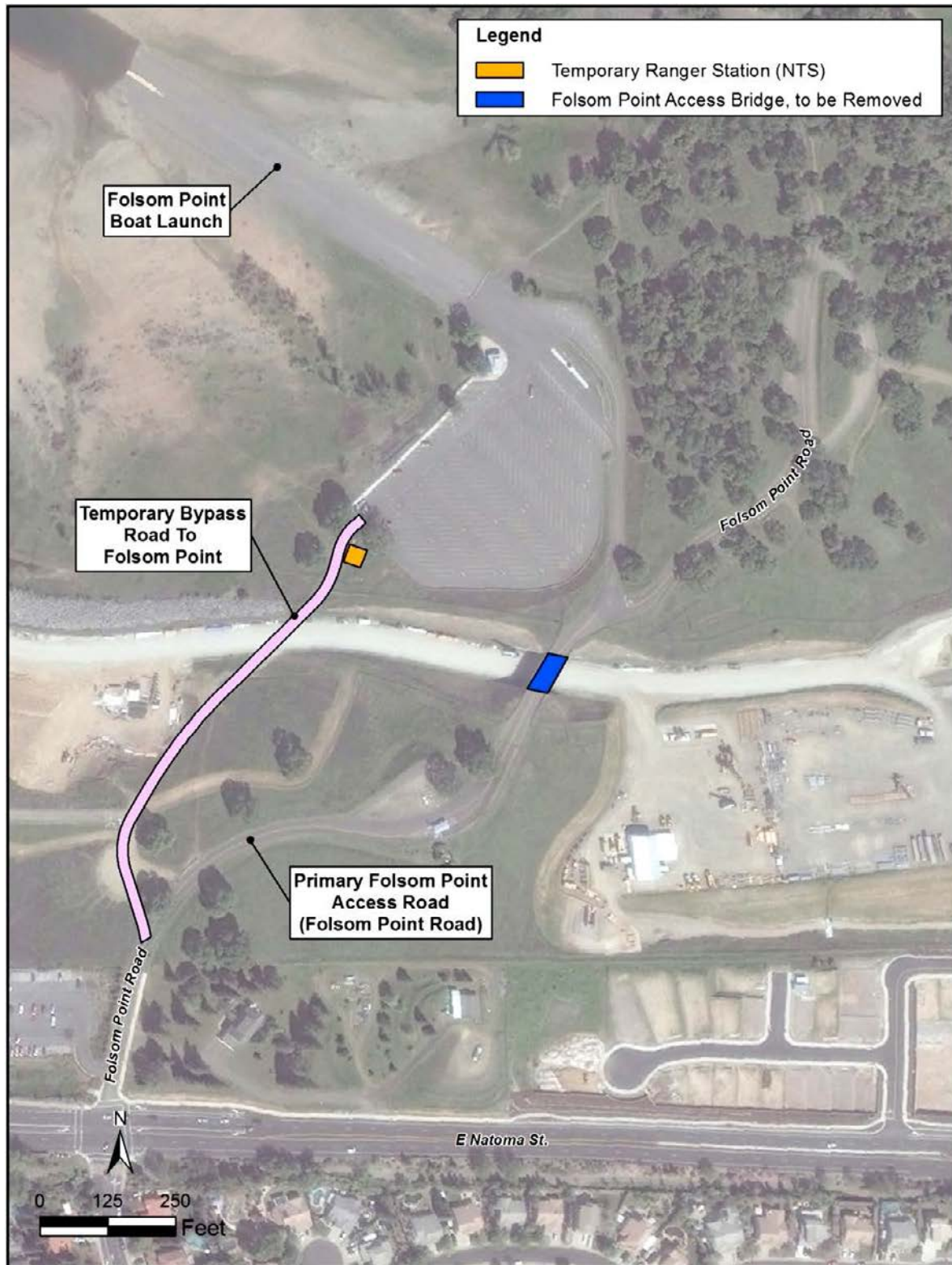
Figure 4. Proposed temporary bypass road to Folsom Point and the existing temporary Folsom Point access bridge to be removed within the Haul Road Restoration Area.
