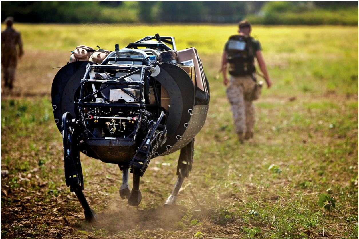
A Marine walks ahead of a legged support system at Marine Corps Training Area Bellows on Oahu, Hawaii. The legged system is designed to carry supplies, including water, food and ammunition, through rough terrain.
