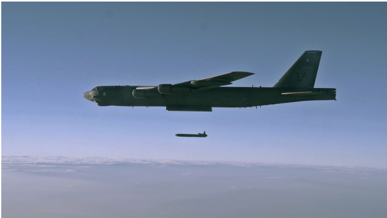
An unarmed AGM-86B Air-Launched Cruise Missile is released from a B-52H Stratofortress over the Utah Test and Training Range during a Nuclear Weapons System Evaluation Program sortie. Conducted by Airmen from the 2nd Bomb Wing, Barksdale Air Force Base, La., the launch was part of an end-to-end operational evaluation of 8th Air Force and Task Force 204's ability to pull an ALCM from storage, load it aboard an aircraft, execute a simulated combat mission tasking, and successfully deliver the weapon from the aircraft to its final target.
