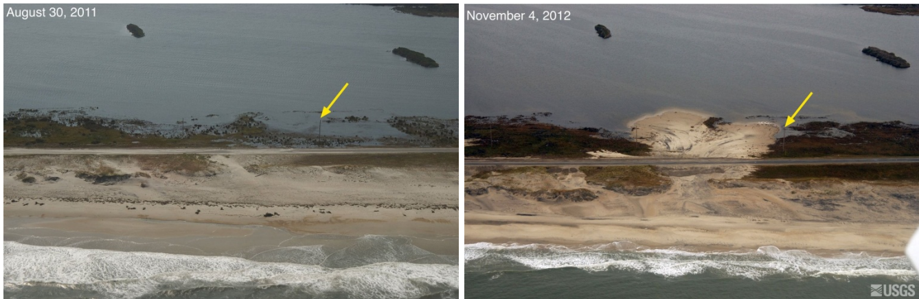
Figure VIII-24. Overwash at the Pea Island National Wildlife Refuge, Kinnakeet, NC (Credit: USGS Coastal & Marine Geology)
