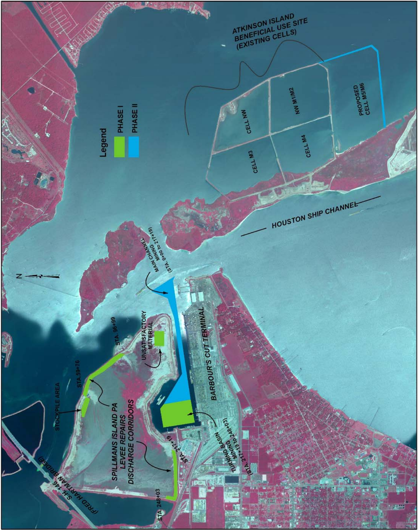
Figure 1. Mining of Barbour's Cut for Spillman's Island Levee Repair and Atkinson Island Beneficial Use Material Site Levee Construction
