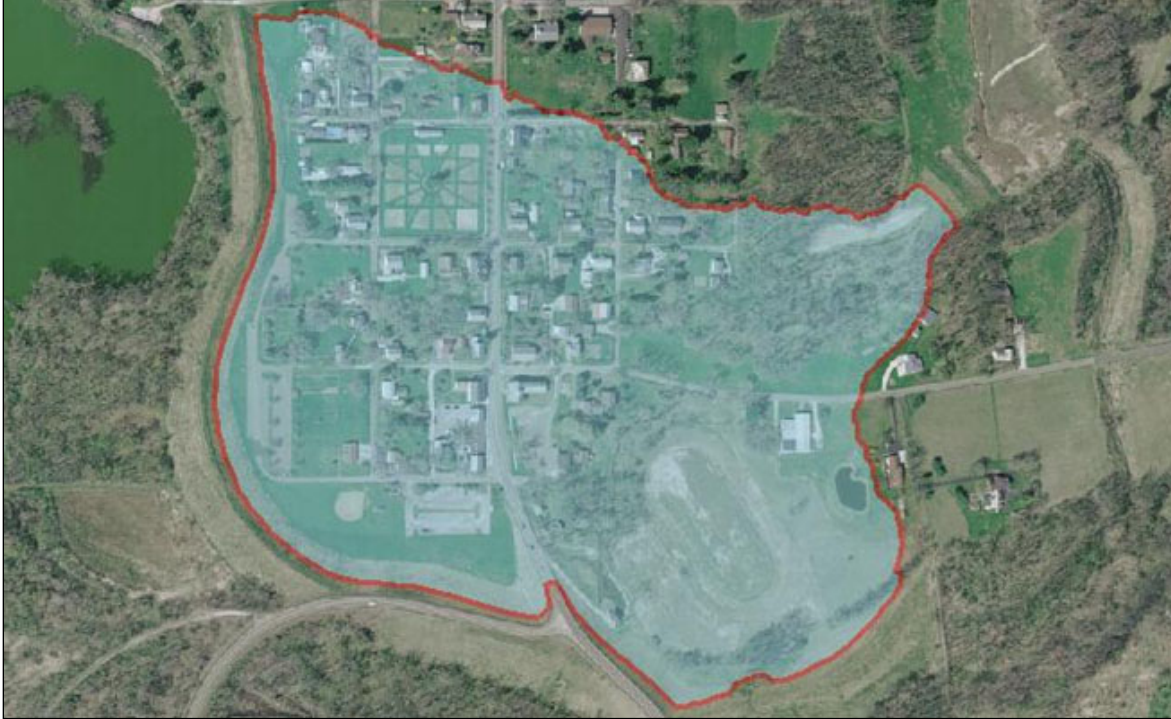
Figure 4. Portion of Zoar Village (shaded in blue) that would be in Dover Dam’s flowage easement of elevation 916’ if it were not for Zoar Levee
