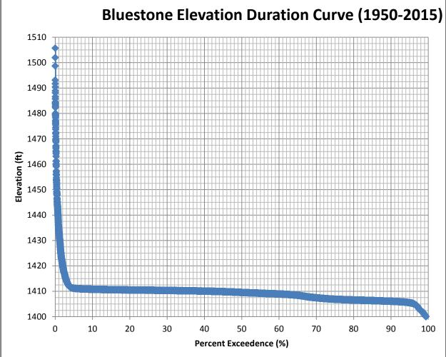
Figure 3: Bluestone Elevation Duration Curve
