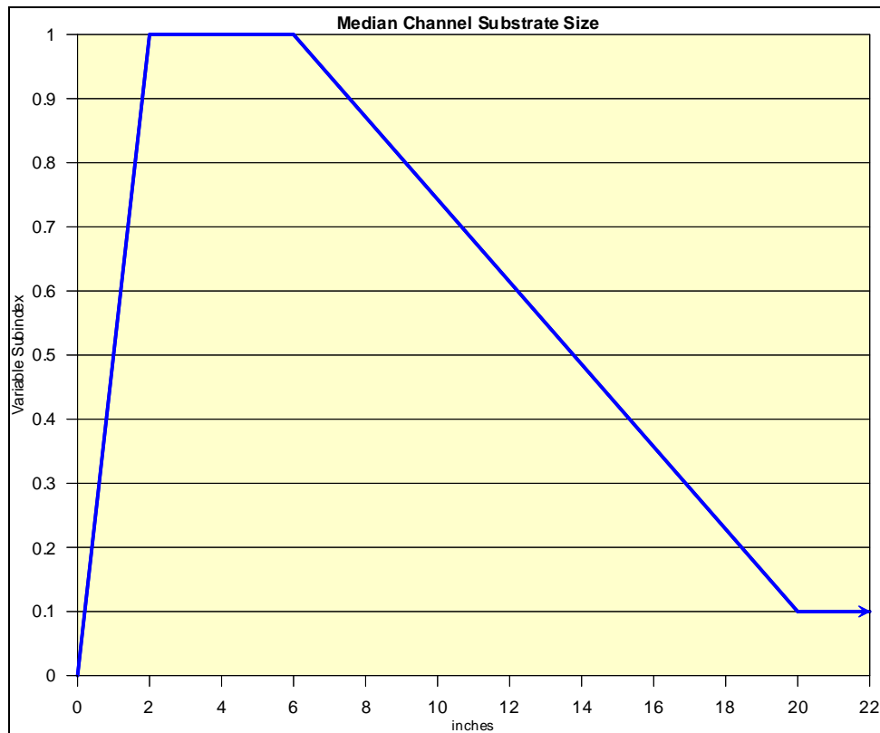
Figure 13. Relationship between median channel substrate size ( V_{SUBSTRATE} ) and functional capacity.
