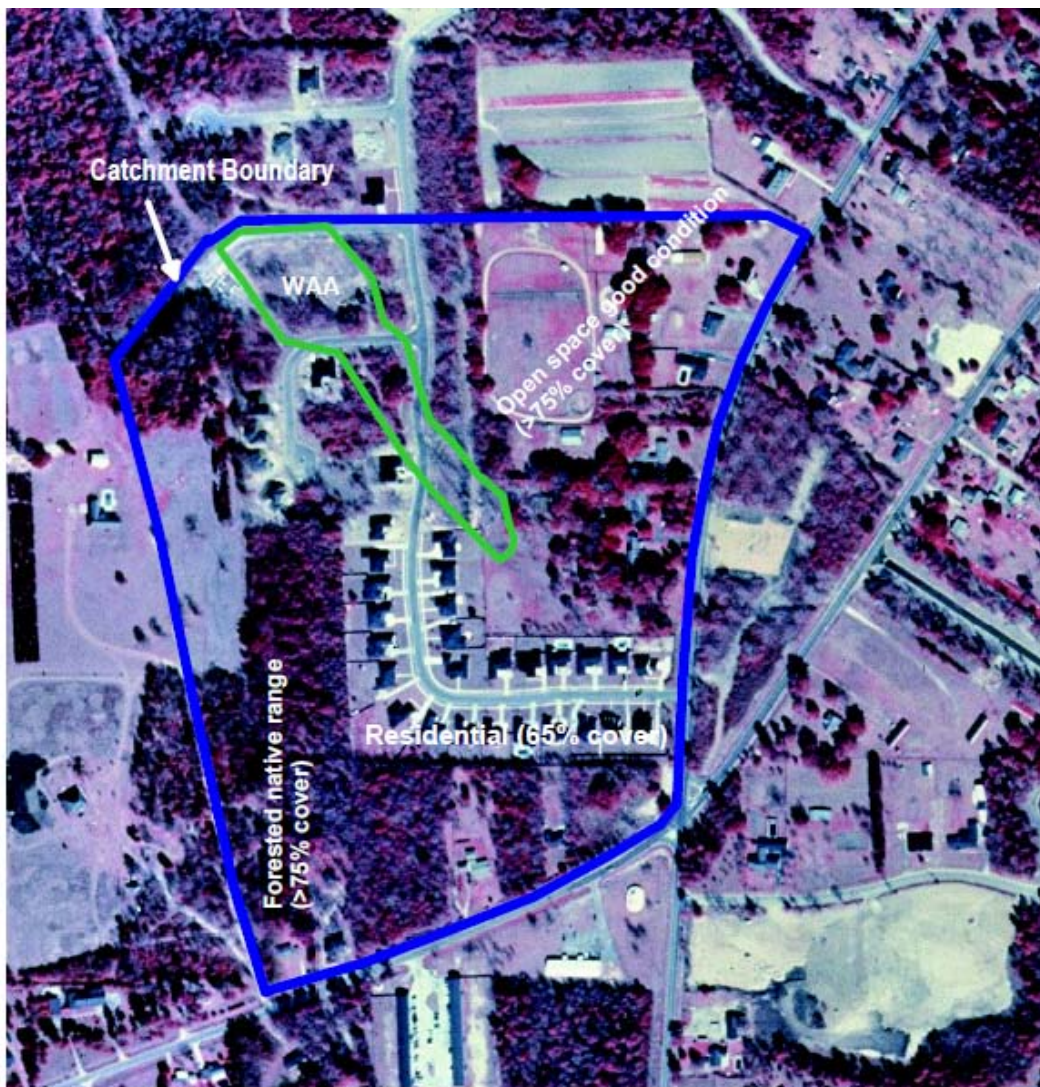
Figure B5. Aerial photograph illustrating the cover types found within a catchment.
