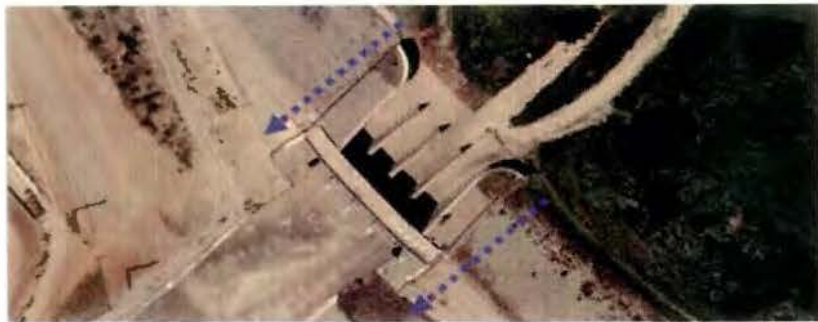
Figure 3: Failure Path for Scour of the Embankment Adjacent to the Outlet Works Wall.
